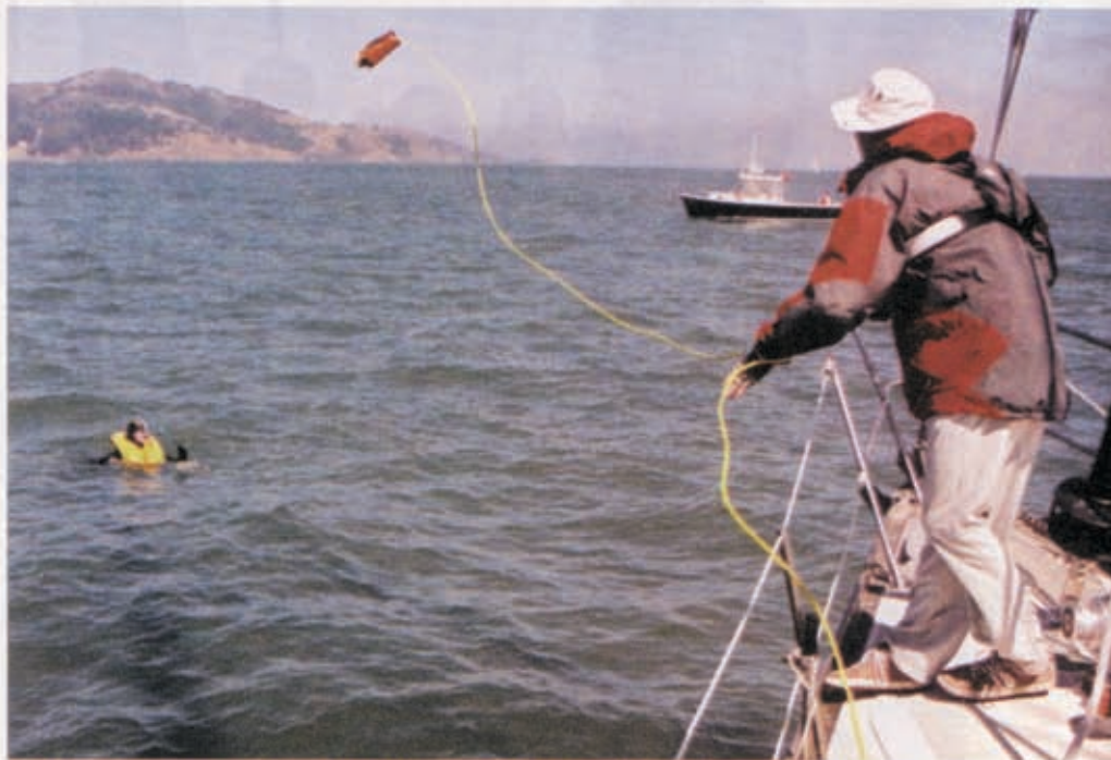
A throwing bag can get the MOB alongside, block and tackle will hoist them
