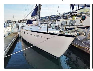
Coho II is MSC's legendary offshore racer/cruiser. She has carried hundreds of MSC students and sailors under the Golden Gate Bridge and onto the Pacific Ocean. At 44.4 feet overall length and 24,000 pounds of displacement, Coho II is built for crossing oceans with speed, seakindly motion, and good performance in both big winds and light airs.
