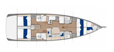
Length overall 14.42 m / 47'4" Hull beam 4.49 m / 14'6" Standard keel draught 2.24 m / 7'4" Fuel capacity 240 I / 63 US gal Water capacity 640 I / 1698 US gal Engines Yanmar 80 HP
