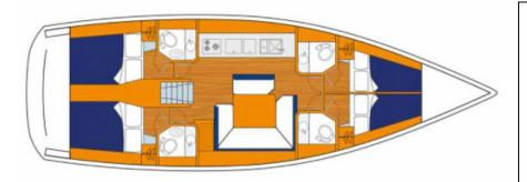
Length overall 14.05 m / 46'1" LWL12.54 m / 41'1" Hull beam 4.5 m / 14'8" Standard keel draught 1.65 m / 5'5" Fuel capacity 240 I / 63 US gal Water capacity 635 I / 168 US gal Engines Yanmar 54 HP
