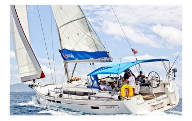
Length overall 14.43 m / 47'4" Hull length13.65 m / 44'9" Hull beam. 4.49 m / 14'8" Standard keel draught 2.24 m / 7'4" Fuel capacity 240 I / 63 US gal Water capacity 615 I / 162 US gal Engines Yanmar 57 HP / 40 KW
